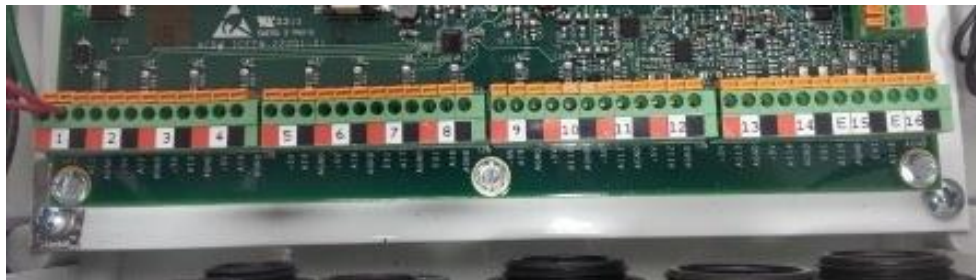
Figure 3. Controller Analog Sensor terminals. See Wiring and Connection Schematic for wiring details.
