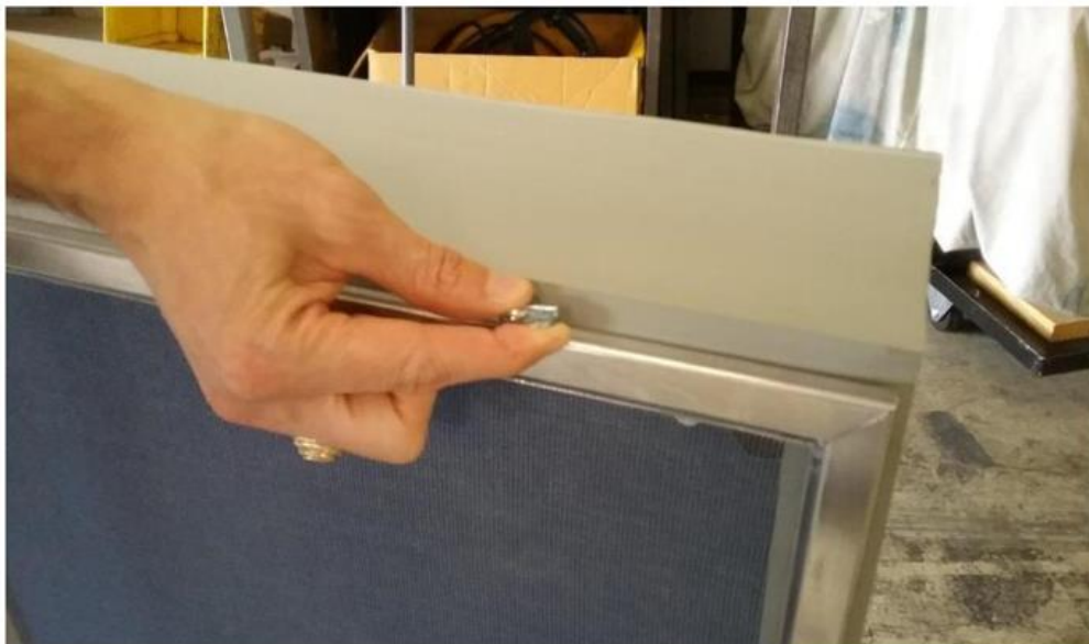
Figure 12. Removal of the screen
