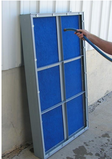
Figure 11. Cleaning the evaporative media with a hose (rear of the EZ-Frame™)
