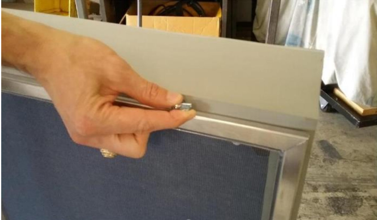
Figure 58. Rotate the latches one at a time to secure the screen in place.
