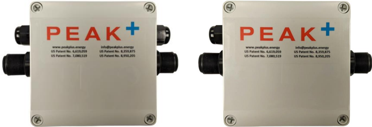
Figure 46. (Above) front view of valve boxes (Left: Junction, Right: Termination)
