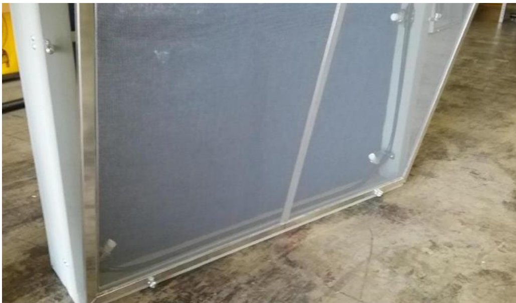
Figure 57. Keeping the bottom latches in an upright position, Tilt and lower the screen into place with the latches.
